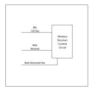
Dimmer has built-in repeater function. Dimmer receives signal from wireless transmitter and rebroadcasts the signal to the next relay receiver.
