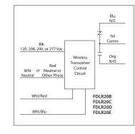
Relay has built-in repeater function. Relay receives signal from wireless switch transmitter and rebroadcasts the signal to the next relay receiver.
