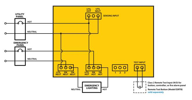
**UL1008 - SWITCH OR 2-WIRE DIMMING APPLICATION**
